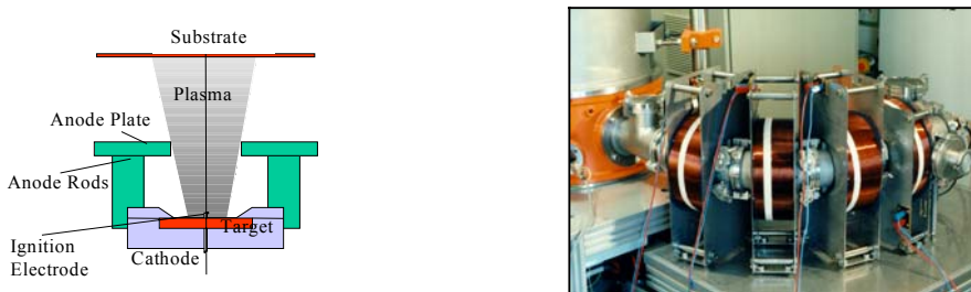
Figure 3.8: Schematic of a pulsed HCA source (left) with magnetic droplet filter (right) (source: FhG IWS Dresden)
