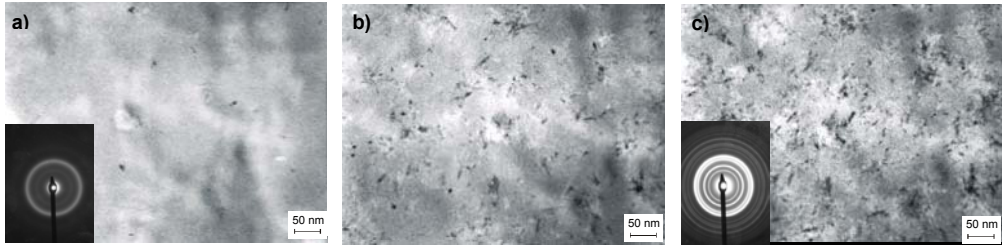
Figure 4.96: Formation of nanocrystals in a \text{ReSi}_{2.22} thin film. TEM micrographs and diffraction patterns of in situ observations during annealing at 630 °C, a) after 5 min, b) after 30 min, c) after 50 min [4.263]
